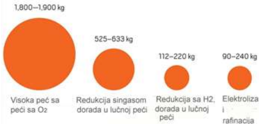
Slika 1 - Poređenje emisije CO 2 po toni gvožđa proizvedenog u klasičnim pećima i pomoću novih tehnologija Figure 1 - Comparison of CO 2 emissions per ton of iron produced in traditional furnaces and using new technologies Izvor / Source: Rechberger et al. (2020), Iron and Steel Technology Roadmap
